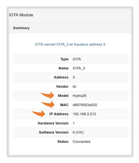
Of interest here is the model, MAC address, and IP address of the AI light. The MAC address is also the serial number of the AI light fixture.
