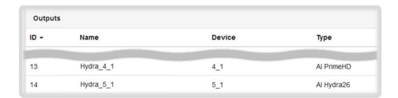
The default output name for any AI IoTa device is model\_#\_1, where *model* may be Prime, PrimeHD, Hydra26, or Hydra52, and # is the Aquabus address of the IoTa module; the AI light model can also be seen in the Type column.
