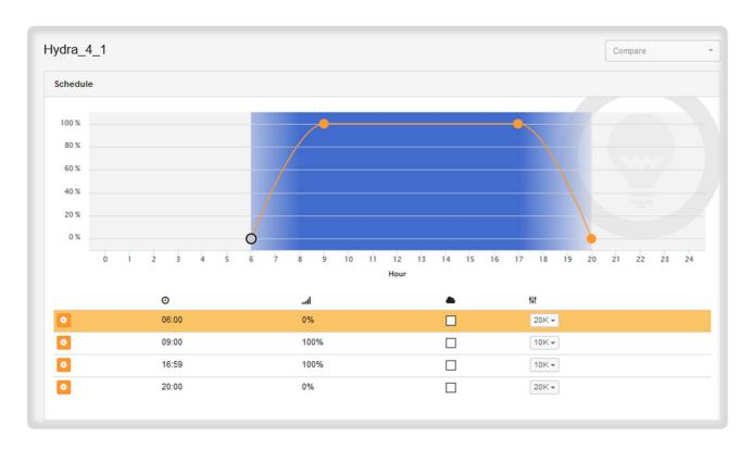
Modify the schedule as desired by dragging each schedule points to adjust the time and overall intensity. Add an additional schedule point by clicking on the \* for a point then
