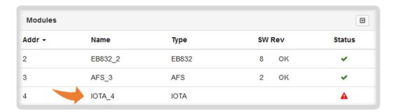
Disregard the lack of data in the **SW Rev** column and the **\( \Lambda \)** in the Status column; this will clear up automatically within a few minutes.
