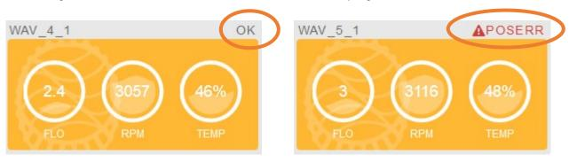
On the WAV tile, a TEMP value equating to the current internal temperature of the WAV is displayed. The normal range of TEMP will be 40-60%.
