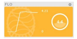
Data from all of the WAVs in your aquarium are aggregated. The size of your tank is factored in, and calculations are done to determine the number of tank volume turnovers per hour, which is then scaled to a FLO number from 0 to 10; the scale is non-linear, similar to the Richter scale used to measure earthquakes. For example, the difference between FLO values of 6 and 7 is much greater than the difference between 2 and 3.
