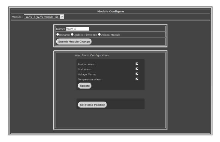
Optionally, the WAV Alarms may also be configured and the Home Position of each WAV set using the display menu.
